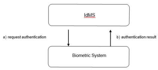
*Figure 3 — Biometric system as an authentication service provider for IdMS*
