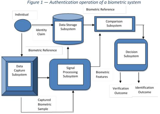
The authentication operation of a biometric system is depicted in Figure 1, to highlight the processing of the identity reference.
